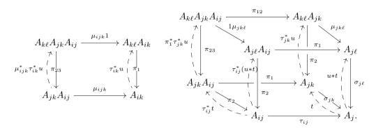
The solid part of the left square is a pullback, and the section to its left obtained by pulling back the one to the right via Lemma 3.17(iii). In particular, the upwards-pointing square commutes, and so we can rewrite u \* (t \* s) as
