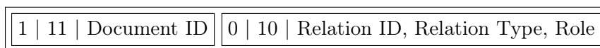
Figure 4.2: Representation of two layers types, one representing Document ID using 3 trailing bytes (binary 11) and the other with relation information occupying two bytes (binary 10)
