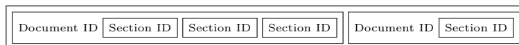
Figure 4.3: Dependent layers such as sections in a document must appear after the document is defined
